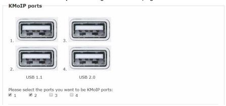
Enable the port #1, 2, 3, 4 for the device to be linked with the TX's K/M over IP HID emulation port. **Default is Port 1 and 2 KMoIP Enabled.**
