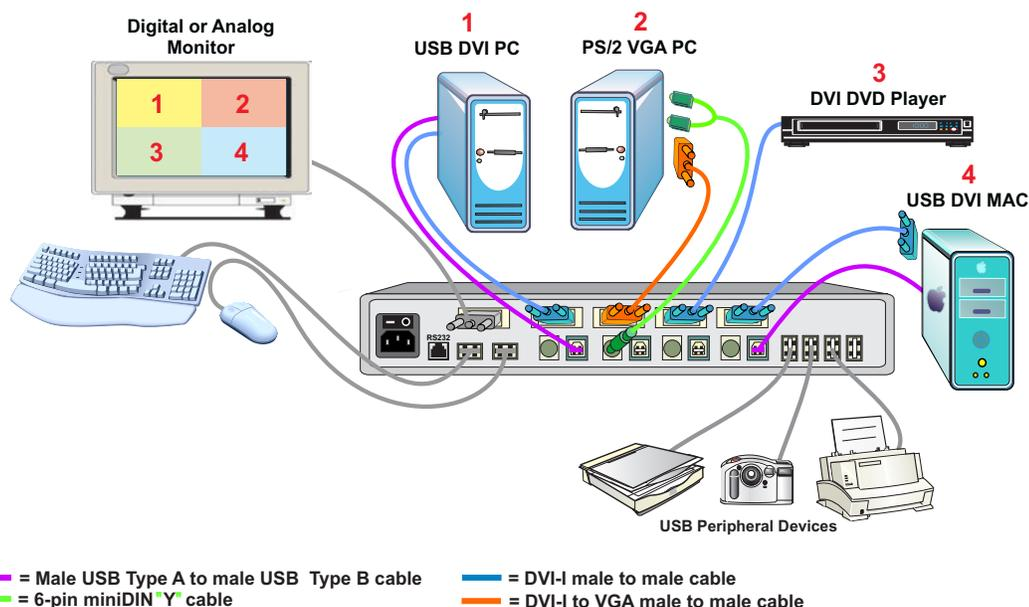
Display video from four computers simultaneously on a single monitor in real time
